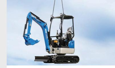
**Arrive quickly at a new place of use:** The lifting eyes integrated in the canopy enable simple and quick moving or loading of the machine by means of the practical two-point suspension.
